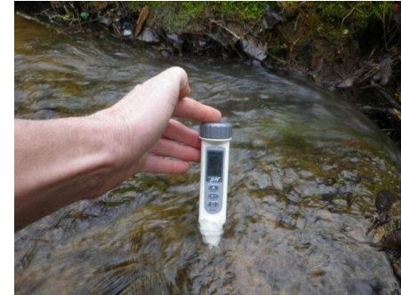
Water quality meter (acidity, temperature, salinity, dissolved oxygen)
